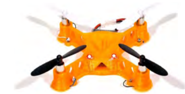
Fig. 7: (a) An 8 bit electronic digital processor with printed-programmable memory by TNO. (b) A quadcopter with included electrical wiring printed by a Voxel8 printer.
