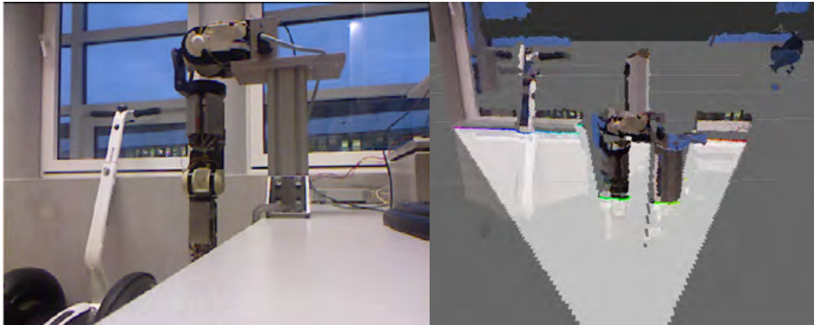
Figure 3: The vision module turns the setting on the left into the data on the right, creating a point cloud and a 2D scan
