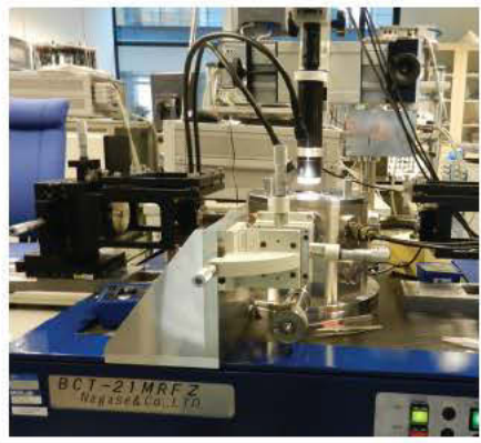
A vacuum chamber with probe station for measurements on piezo actuated resonators.
