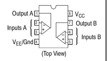
The polarization is given using a dot on the first pin, the small notch also denotes the side with pin 1. The chip contains two OpAmps and requires a supply voltage of at least 5V
