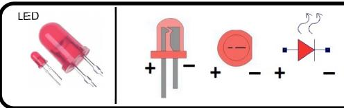
Note polarity! Also use a series resistor. LED 's can take 20mA. In most cases 330R is good enough.
