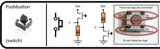
A switch can be connected using a 10k pull-up resistor. (or pull-down) You might have to straighten the legs to t the breadboard
