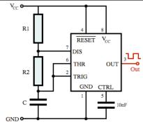
Versatile timing chip. Can be used to make oscillators, PWM generators, delay timers etc. In this circuit:
