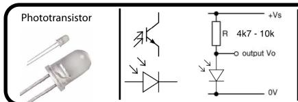
Note polarity. The same markings used with an LED apply, although the wire length is different. A phototransistor or photodiode conducts current depending on received light intensity. Use a pull-up resistor.
