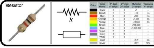
Resistors do not have polarization. Colored rings are used to denote the value. Ohm 's law applies: V=I\*R
